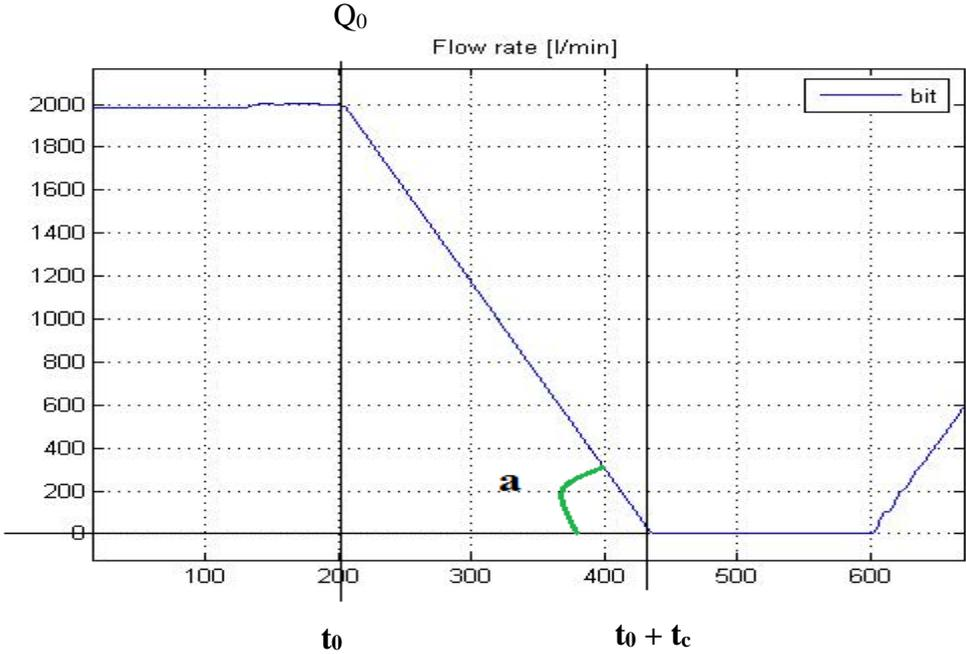
Figure 1 Shutdown flow rate example. From 2000 to 0 l/min over time interval [t0, t0+tc]
