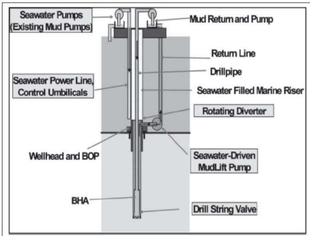
Figure 3.5 Subsea Mudlift Drilling arrangement<sup>[10]</sup>
