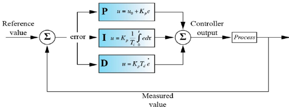
**Figure 7.2 PID Controller<sup>[2]</sup>**
