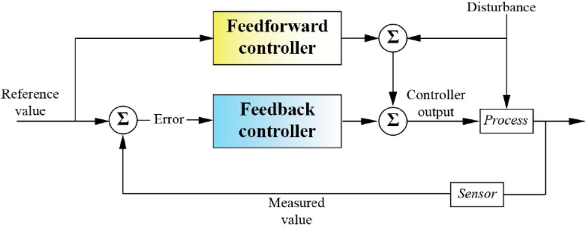
**Figure 7.3 Feedforward Control<sup>[2]</sup>**
