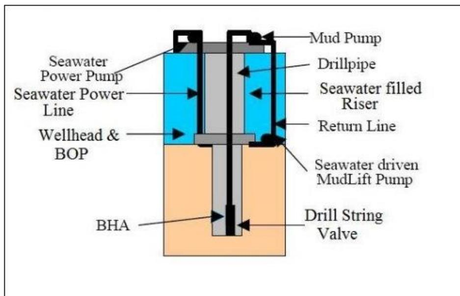
**Figure 2.2. Simple overview of DGD components<sup>[10]</sup>**
