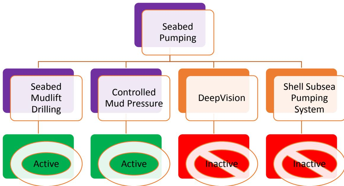
**Figure 3.3 DGD methods under the Seabed Pumping classification.**
