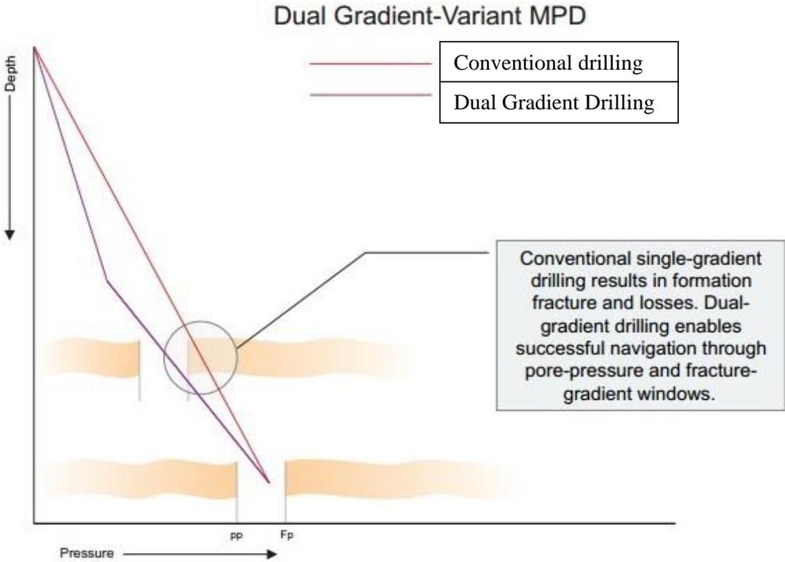
**Figure 2.1: Pore pressure and fracture pressure gradient in Conventional drilling vs DGD<sup>[9]</sup>**
