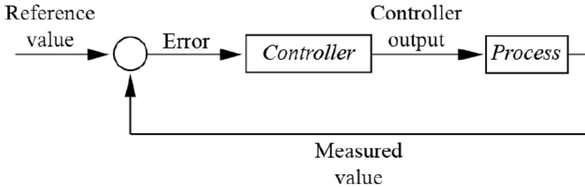
**Figure 7.1 Linear error control<sup>[2]</sup>**
