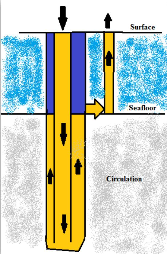
Figure 5.4 U-tube effect in closed system<sup>[30]</sup>
