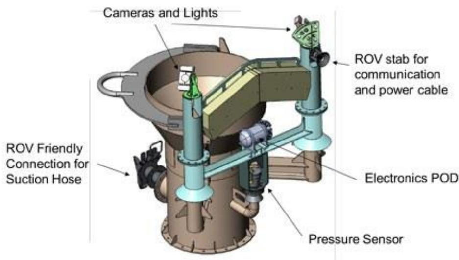
**Figure 4.3 Suction Control Module<sup>[16]</sup>**
