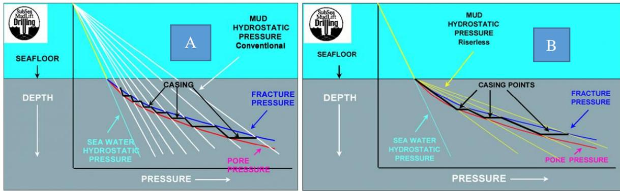
Figure 5.1 A - Conventional Casing Requirements. B - Riserless Casing Requirements<sup>[29]</sup>
