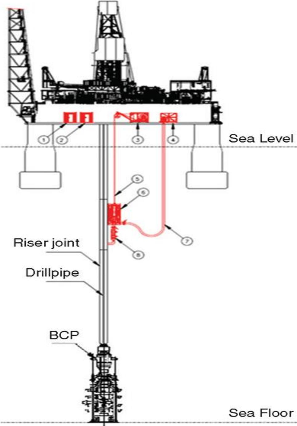
Figure 3.6 Typical EC-Drill setup <sup>[19]</sup>
