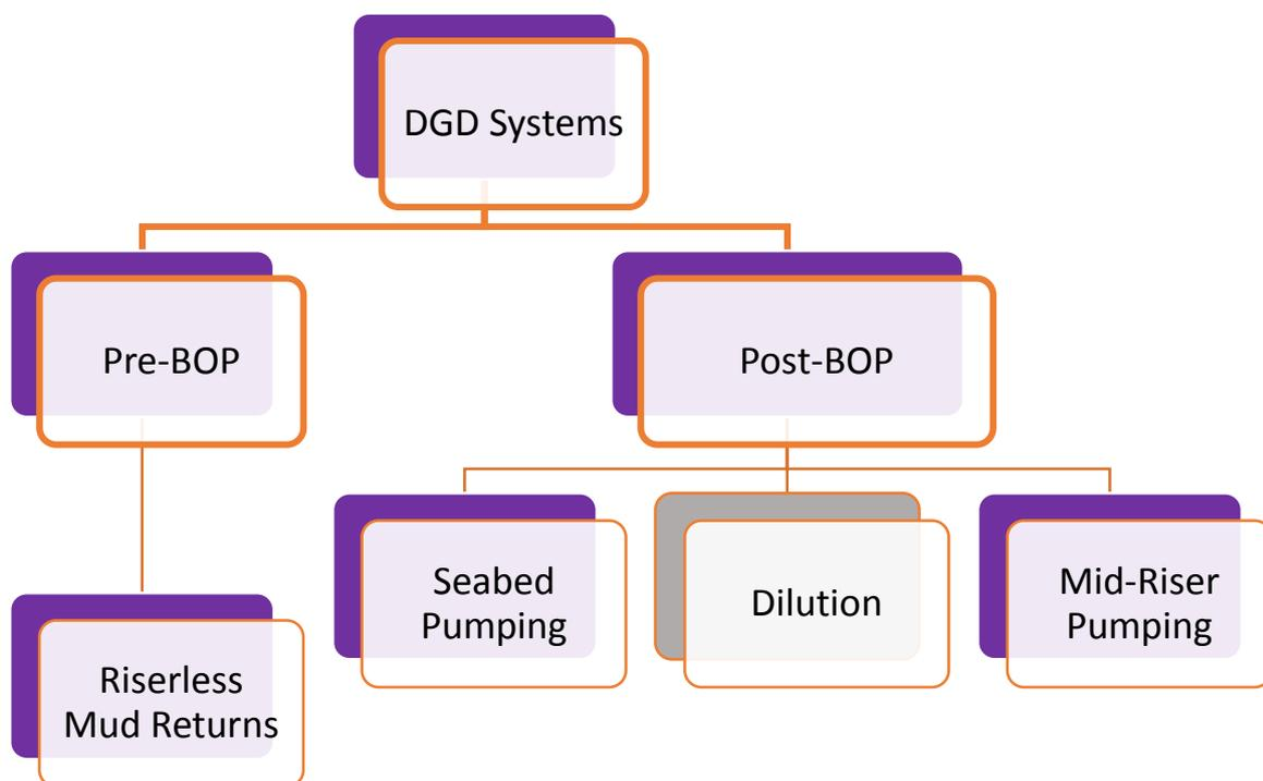
Figure 2.3. Dual Gradient Drilling Classification tree
