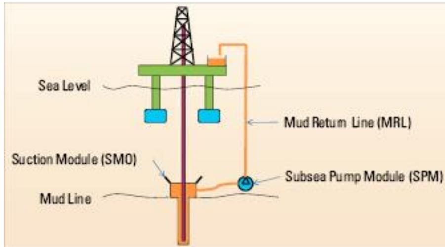
**Figure 3.1 Riserless mud recovery uses a subsea pump module located near the seabed to pump fluid and cutting returns from the well to the rig mud-treatment system via the Return Line.<sup>[16]</sup>**
