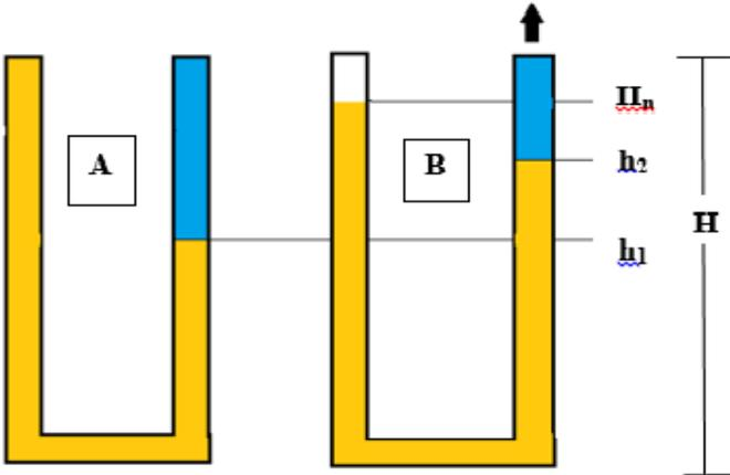
**Figure 5.2 Simple illustration on the u-tube effect in an open system. The figure is missing some information: Left column – drill pipe, right – annulus, BHP and parameter description. The heavier mud in beige and the lighter in blue. A: Imbalance of pressure. B: Mud freefall, U-tubing.<sup>[30]</sup>**
