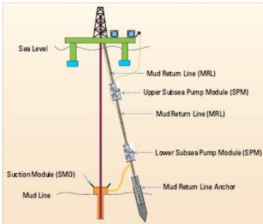
**Figure 3.2 Deepwater RMR uses an anchoring system to keep the Return Line from swinging into the drill string.<sup>[16]</sup>**
